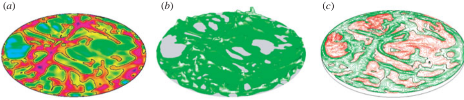
FIGURE 5. Results for the constant-heat-flux condition at the lower plate, Ra_q = 2 \times 10^{11} , ( Ra = 2.22 \times 10^9 ) Pr = 0.7 . (a) Instantaneous temperature distribution at the lower plate: thick —, \theta = \bar{\theta}_w ; blue, magenta and red, \theta > \bar{\theta}_w ; yellow, green and cyan, \theta < \bar{\theta}_w . (b) Perspective view of the instantaneous temperature isosurface ( \theta = 0.8\bar{\theta}_w ) close to the lower plate. (c) Contour lines of vertical velocity at a distance of \approx 0.015h from the lower plate; green and —, positive velocities; red and ·····, negative velocities.
